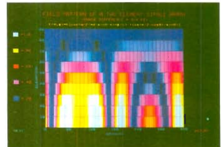
Electromagnetic energy values are represented by a color scale on the System 45C.
